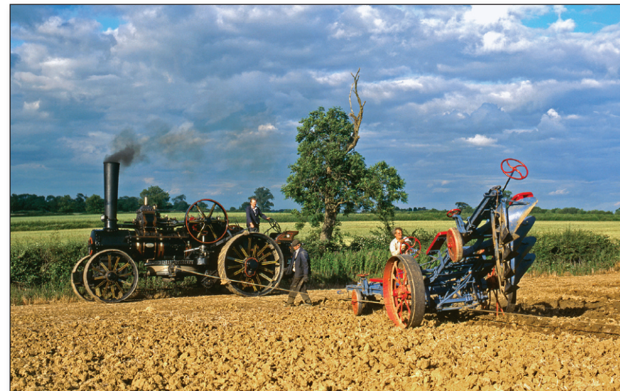
On a beautiful summer afternoon in rural Warwickshire, Fowler AA7 Ploughing Engine No. 15257 built in 1918 simmers as the four furrow balance plough sets off across the field winched by the second ploughing engine.
