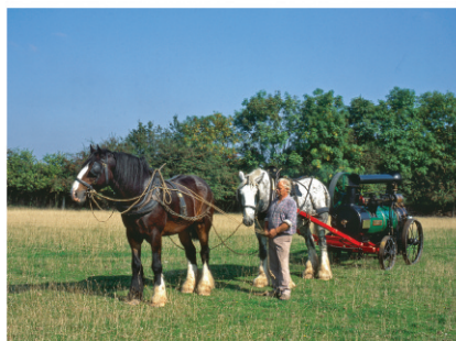
A demonstration of how the diminutive 1866-built Brown & May Portable Engine would have traditionally been moved around using horse power. Note how the chimney has been folded down to improve stability.
