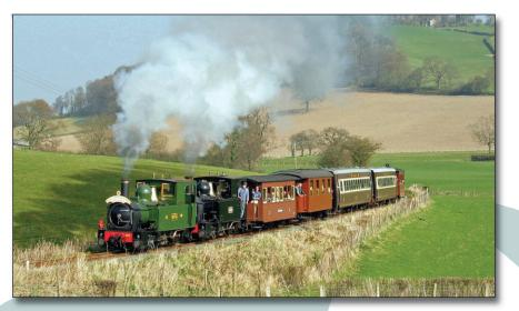
Beyer Peacock supplied two 0-6-0Ts for the 1903 opening of the 2ft 6in gauge Welshpool & Llanfair Light Railway, one of the few narrow gauge branch lines to be built under the 1896 Light Railways Act. A Centenary Special working on 5 April 2003 sees No 1 The Earl and No 2 Countess climb towards Coppice Lane crossing.
