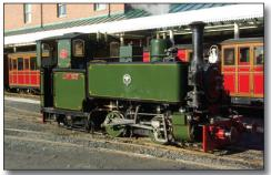
1949, 1991 — This 0-4-2T is a new locomotive 'by the back door'. Tom Rolt, named after the founder of the Talyllyn Railway Preservation Society, was built at the line's Pendre Works, incorporating components of a little-used 3ft gauge Andrew Barclay 0-4-0WT built in 1949 for Bord na Mona (the Irish Turf Board) nicknamed Irish Pete.
