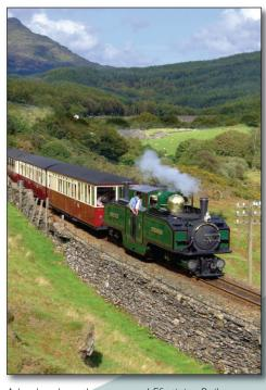
A landmark on the preserved Ffestiniog Railway came in 1979 when, 110 years after Little Wonder appeared on the line, a brand new double Fairlie, Earl of Merioneth, based on the original patent, although with modern box-like side tanks, emerged from Boston Lodge Works.
