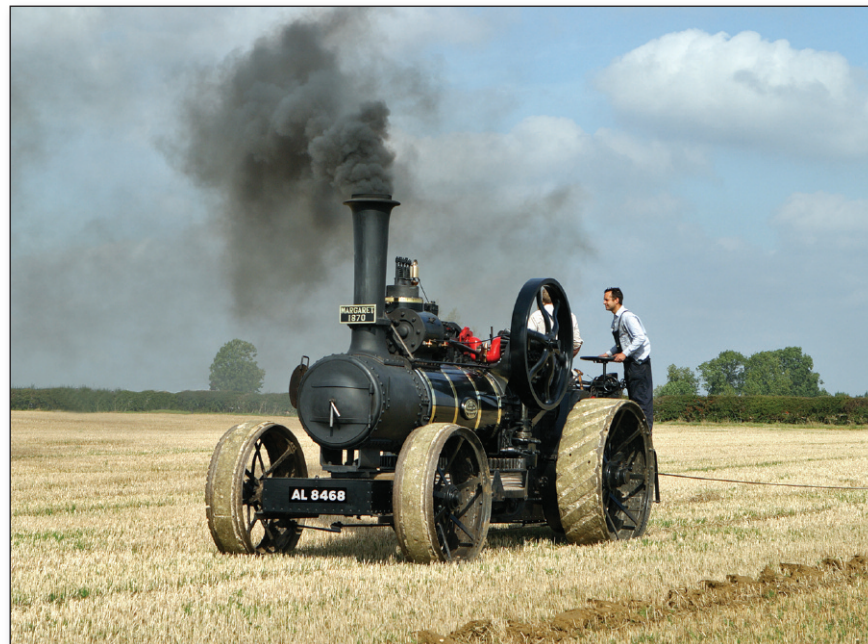
The second oldest preserved Fowler engine in the UK, 'Margaret', a single cylinder 12NHP ploughing engine built in 1870.
