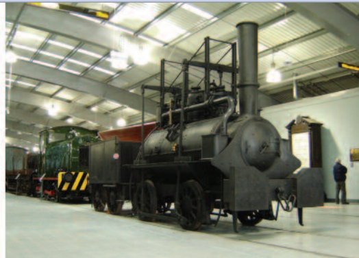
In 1845, 2-2-2 No 49 Columbine became one of the first locomotives to be built at the Crewe Works of the Grand Junction Railway, the world's first trunk railway when it opened in 1837. Columbine ran until 1902 and is now in the Science Museum.
