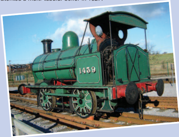
London & North Western Railway 0-4-0 saddle tank No 1439, built in 1865, is now on display at Locomotion in Shildon.
