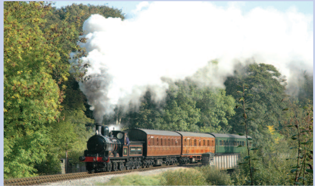
Perhaps best known as The Green Dragon in the EMI big screen production of Edith A Nesbit's classic The Railway Children, Lancashire & Yorkshire Railway Class 25 0-6-0 tender locomotive No 957 designed by Chief Mechanical Engineer William Barton Wright. Built by Beyer Peacock in Manchester, the type became known as 'Ironclads'.
